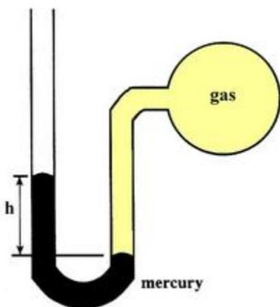
Atmospheric pressure is 749 mmHg. What is the pressure of the trapped gas? ( $h = 29.2 \text{ cm}$ )
